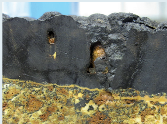
Sample from approximately 1,700 metres water depth from a seamount of the Louisville chain in the southwest Pacific. The crusts from this region contain up to 1.6 percent cobalt and are significantly enriched in rare earth elements, molybdenum and titanium. Photo: BGR
