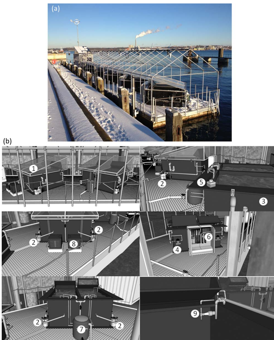
Fig. 2. (a) Overview of the Kiel Outdoor Benthocosm infrastructure showing the six tanks with their subunits covered by hoods as well as (in the background) the technical container bearing on its roof the solar panels and the wind generator. (b) Sketches of important functional components of KOB. Not shown are the numerous IT components. 1: hood, 2: circulatory pumps, 3: position of lateral ports, 4: measurement cell, 5: pCO 2 sensor, 6: measurement and control unit, 7: heat exchanger, 8: coolers, 9: water inflow (and air injection (not shown)).
