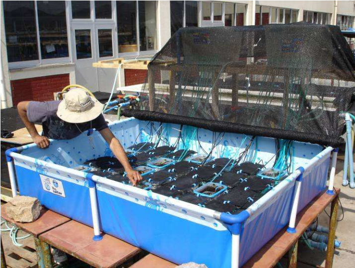
Figure 2: Outdoor set-up used for the manipulation of light availability for macroalgae. Coquimbo, Chile 2007. Photo: Christian Pansch
