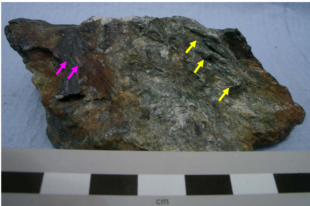
Fig. 2. Sample 310ROV-2. Serpentinite; strongly foliated and internally sheared; note the formation of micro-phacoids (yellow arrows) with orientation along the striations visible on the surface of the rock (pink arrows)
