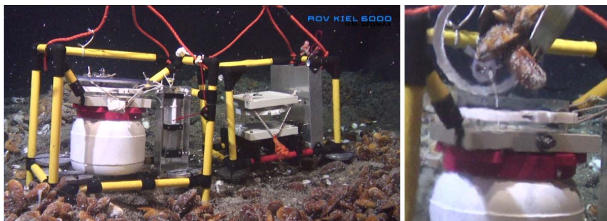
Fig. 2.4.8.1: In situ fixation chambers. Left: DieFasts 1 (right) and 2 (left) sitting on the seafloor in “Clueless”. Left: Loading of mussels into a seawater-filled top chamber of DieFast 2. After closing the top lid, a trapdoor opens and the mussels slide down into the RNA Later-filled main chamber (white drum). The two-chamber design was chosen to minimize mixing of the saturated RNA Later solution with seawater during the loading with mussels.
