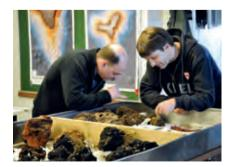
Investigation on board: In the wet laboratory of the research vessel POSEIDON, the rock samples of an active underwater volcano that were collected with the submersible JAGO are inspected. Photo: Maike Nicolai/GEOMAR
