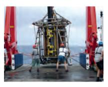
**Rockdrill 2,** a drilling rig of the British Geological Survey, is capable of drilling through hard rock down to 15 metres and is deployed directly at the seabed. Here, the core is drilled in 10 1.5-meter long sections. Source: GEOMAR
