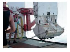
Video-guided grabs are equipped with a camera inside that sends real-time videos to the ship via a deep-sea cable. This allows the shovels to be closed in a controlled manner and rock samples to be taken. Photo: Sven Petersen/GEDMAR
