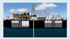
4: On the vessel, the ores are separated from seawater and sediment and transported to the storage tanks.
