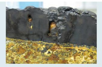
Sample from approxiamtely 1,700 metres water depth from a seamount of the Louisville chain in the southwest Pacific. The crusts from this region contain up to 1.6 percent cobalt and are significantly enriched in rare earth elements, molybdenum and titanium. Photo: BGR
