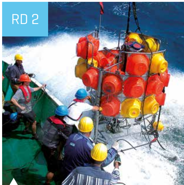
Biogeochemical observatory: BIGO-landers are used for the study of exchange processes between sediment and water column. Image: GEOMAR
