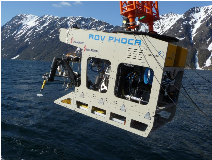
Figure 2: ROV “PHOCA” carrying an Eddy Correlation Module on the front porch ready for deployment.
