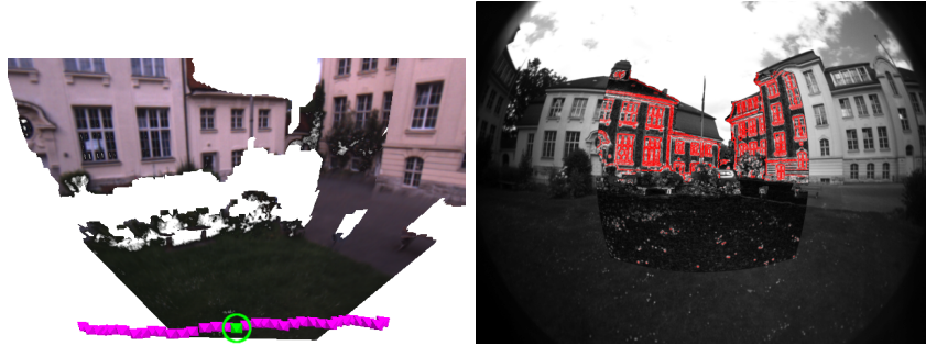
Figure 6.13: Top: Perspective view onto reference model School from above and extent of camera movement used for drift measurement. The camera is going forward/backward from one end of this path to the other. It passes the green middle camera, where the pose estimation is compared to previous and following passes (see table 6.2). Bottom: augmentation of model view and real image using estimated parameters. The texture used for the augmentation is the gradient magnitude of original texture, strong gradient edges colored in red.
