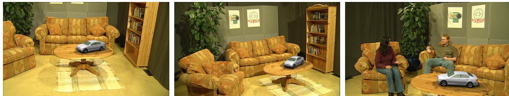
Figure 6.1: A virtual car model inserted into a scene. When the camera is tracked, virtual 3D models can be overlaid such as if they were in the scene.
