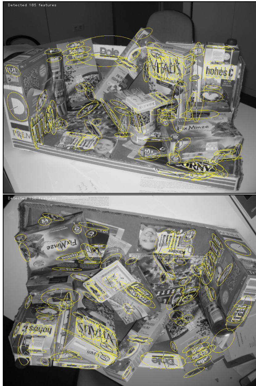
Figure 4.2: Two images with wide baseline, where the camera was additionally rolled by 180^\circ . In these images MSER[Matas et al., 2002] features have been detected as indicated by the small ellipses. The ellipses represent the mean and the second central moment of the pixels segmented by the watershed algorithm.
