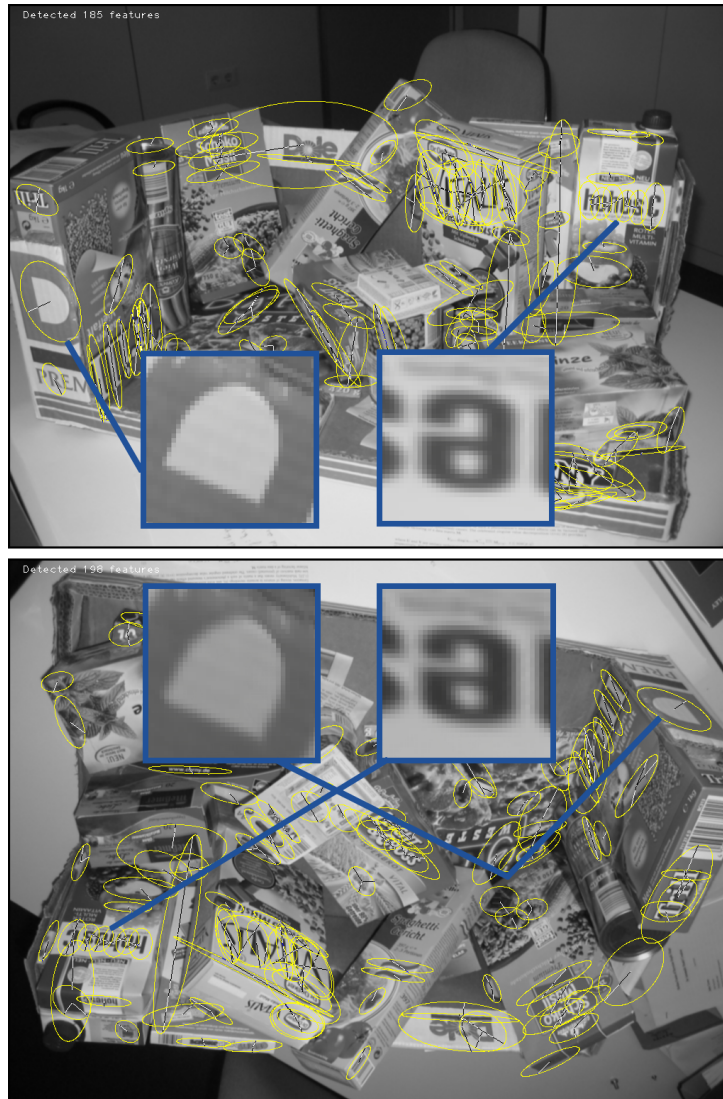
Figure 4.3: In each of the MSER features from figure 4.2 the local gradients have been exploited to obtain a main orientation as proposed by Lowe[Lowe, 2004]. Together with the elliptical shape this provides a full affine coordinate system, the local affine frame. Two features are shown in their LAF coordinate system (after optimization). As can be seen, this normalization results in two almost identical local regions. This means that a concatenation of the two transformations warps the local region of the first image onto the local region of the second image. Mathematically, this transformation is the linearization, or the first order Taylor approximation of the true homography.
