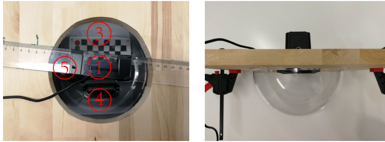
Fig. 8. Experimental settings of the webcam with an acrylic dome. Left: Top view with test positions, Right: Side view.
