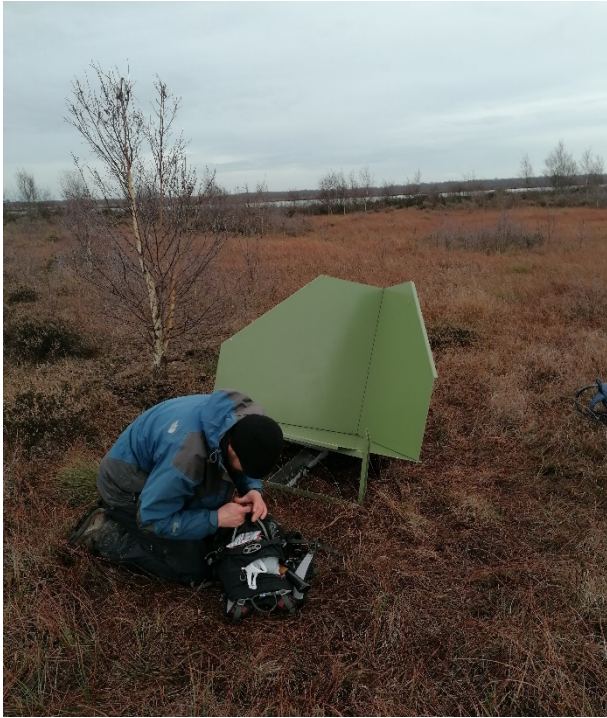
Fig. 5. One of the corner reflectors placed at the Hatfield Moors natural gas storage site
